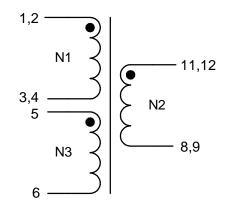
Application of the transformer allows for the leadwires between terminals 1&2, 3&4, 11&12, and 8&9 to solder bridge.
