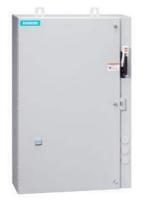
Non-reversing motor starter Size 2 1/2 Three phase full voltage Solid-state overload relay OLRelay amp range 25-100A 240V 50HZ / 277V 60HZ coil Combination type 100A circuit breaker Enclosure NEMA type 4/12 Water/dust tight for outdoors Standard width enclosure
