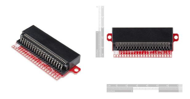
**Description:** The SparkFun micro:bit Breakout is a board that connects to the BBC micro:bit and expands the capabilities of the development platform by providing access to more pins and allowing for connections to the I<sup>2</sup>C and SPI buses. This breakout board for the micro:bit's edge connector allows intermediate and advanced users to connect the micro:bit to breadboards and other sensors, motors, LEDs and more!
