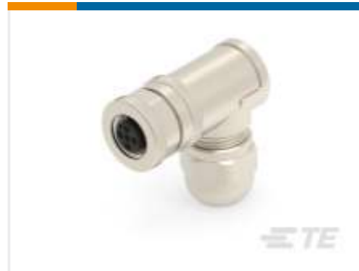
TE Part #T4112012041-000 M12 F, 4P GOLD A_CODE RA SHIELDED PG9
