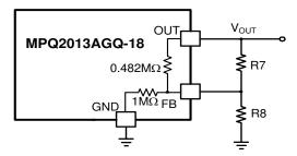
To lower the additional current dissipation, resistors of FB divider on the demo board are chosen to high value. If part would performance no load when Ta>85°C, FB dividers should be lower to maintain a minimum load to draw the leakage current from OUT pin. The recommended maxim value of R8 is  $1M\Omega$  when Ta≤105°C and  $210k\Omega$  when Ta≤125°C. Once R8 is determined, R7 can be calculated by below formula:
