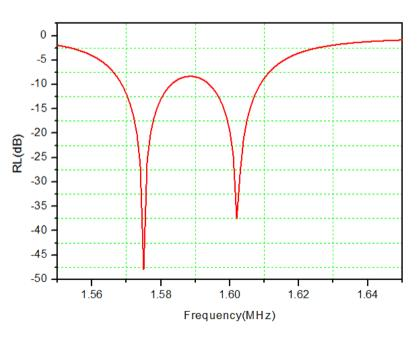
Return Loss characteristic shows a dual band response for GPS/Galileo & GLONASS
