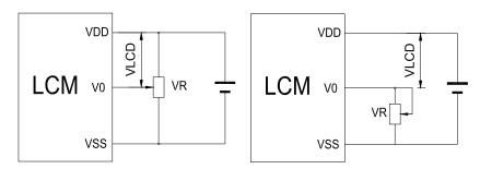
VDD~V0: LCD Driving voltage
