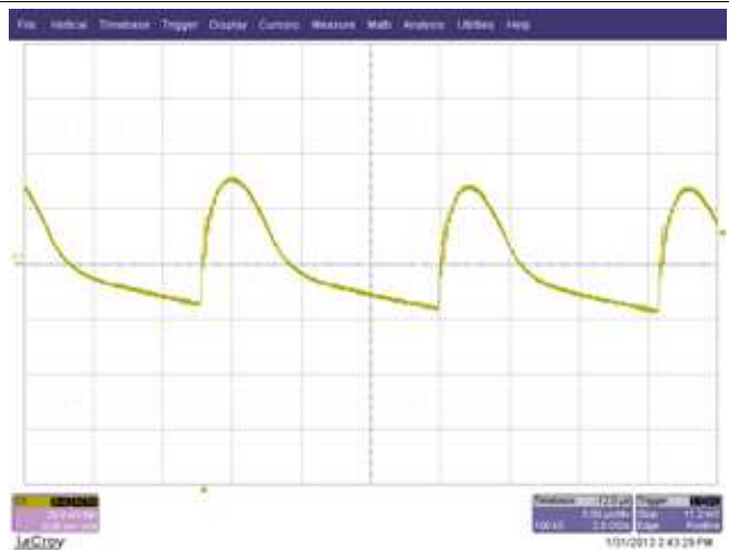
Figure 46. Ripple with 5-V, 1.2-A Output, 265- V_{AC} Input, 20 mV/div 5 \mu s/div
