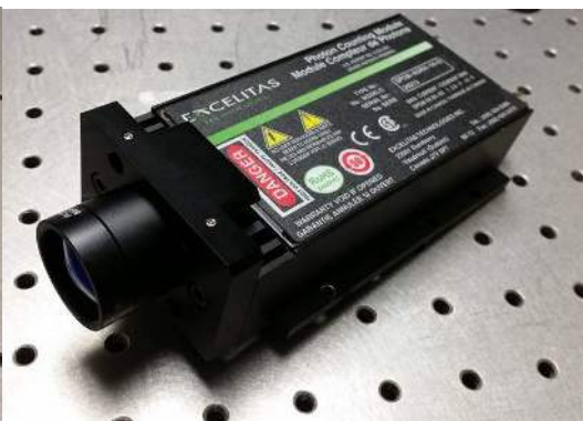
SPCM-AQRH-WX-BR2: with bracket for C-mount (1.0" x 32TPI) and 30mm cage mount
