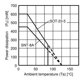
Figure 5 Power Dissipation of Package (Mounted on Board)
