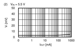
3. 3  $V_{OUT} = 3.3 \text{ V } (R_{FB1} = 36 \text{ k}\Omega, R_{FB2} = 8 \text{ k}\Omega)$
