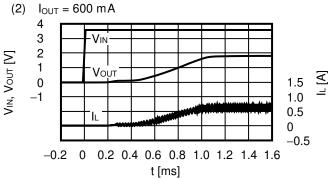
3. 2 Shutdown pin response ( $V_{OUT} = 1.8 \text{ V}$ ,  $V_{IN} = 3.6 \text{ V}$ ,  $V_{ON/\overline{OFF}} = 0 \text{ V} \rightarrow 3.6 \text{ V}$ ,  $Ta = 25^{\circ}\text{C}$ )
