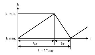
Figure 10 Continuous Mode (Current Cycle of Inductor Current (I<sub>L</sub>))
