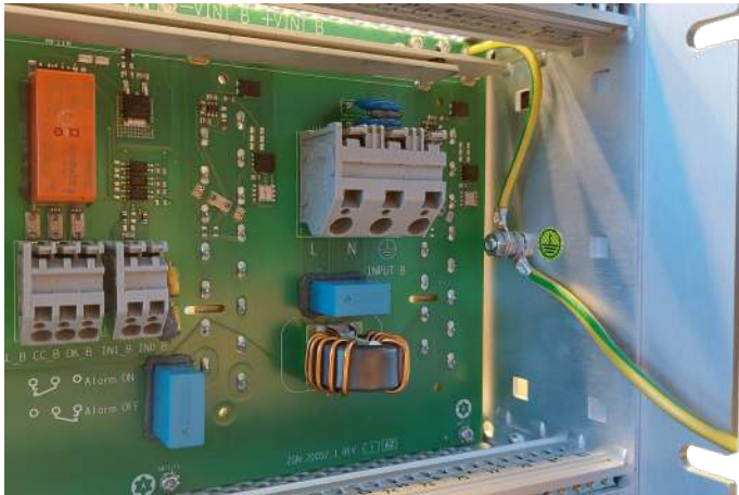
Fig. 8 Protective earthing of LRSA subrack system
