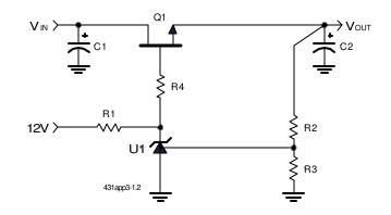
Figure 3- Low cost 3.3V to 2.7V output for Intel I740 application.
