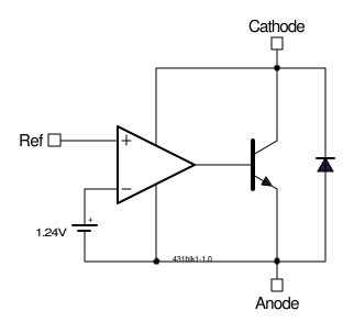
Figure 1 - Simplified block diagram of the IRU431L
