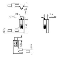
This cable includes a 10K pullup resistor between the 'CC' line and 'V<sub>BUS</sub>'. For systems compliant with the USB Type-C Cable and Connector Specification, the cable current will be restricted to 3.0A.
