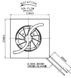
Marking (By laser): SUNON UB3H3-700 TC:Model name Production serial number:0Y17xxxxxx 0:Printing Plant Code Y:Manufacture Plant 17:Year,2017=17 xxxxxx: Producing Lot No. QR code :Content according to SUNON QR code specification TC:CUSTOMER NUMBER
