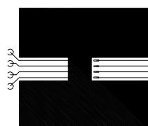
a)  $50^\circ \text{C/W}$  when mounted on a  $1 \text{ in}^2$  pad of 2 oz. copper.
