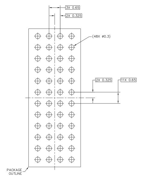
PCB DESIGN GUIDELINES - I/O PADS AND SOLDERABLE AREA
