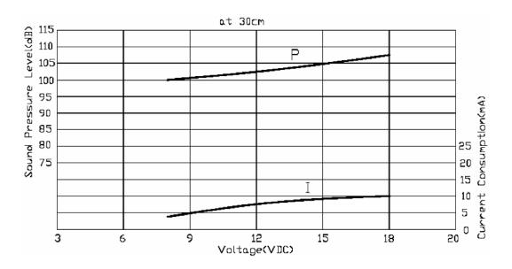
P: Voltage vs. Sound Pressure Level I: Voltage vs. Current Consumption
