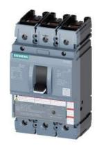
circuit breaker 3VA5 UL frame 250 breaking capacity class M 35kA @ 480 V 3-pole, line protection TM230, FTAM, In=200A overload protection Ir=200A fixed short-circuit protection Ii=5...10 x In cable connection on both sides
