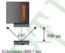
To be measured at the center area of panel with a viewing cone of 1° by Topcon luminance meter BM-7, after 10 minutes operation (module)
