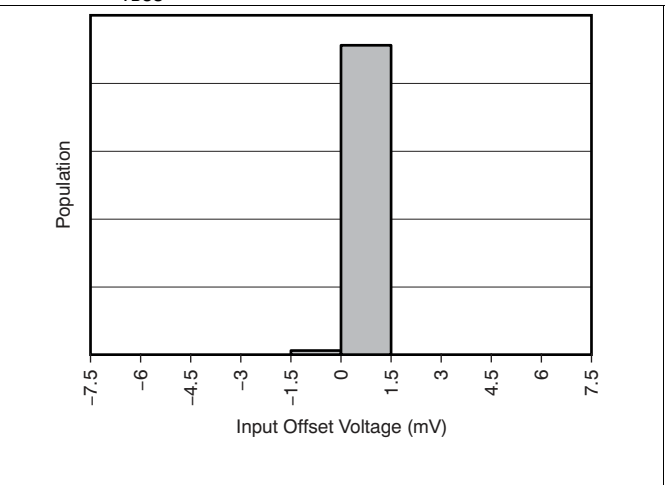
Figure 8. Bus Input Offset Voltage Production Distribution
