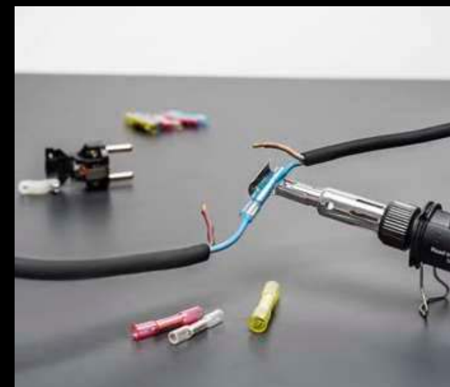
Create an even seal on solder sleeves
