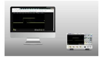
With the new embedded web server, users can control the oscilloscope from a simple web page. This provides wonderful remote troubleshooting and monitoring capabilities.
