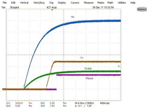
Fig. 7: Start up at 12A Load Ch 1 :V out , Ch 2 :V in , Ch 3 :PGood, Ch 4 :Enable
