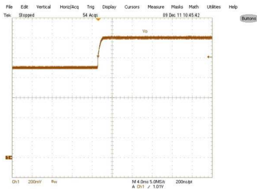
Fig. 9: Start up with Pre Bias , 0A Load, Ch 1 :V o
