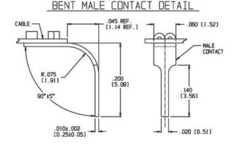
ALL DIMENSIONS: INCHES [MILLIMETERS] ALL TOLERANCES: ±0.005 [0.13] UNLESS OTHERWISE SPECIFIED MAY SHIP WITH OR WITHOUT POLARIZATION STRIPE UNLESS SPECIFIED CONSULT FACTORY FOR OTHER SIZES AND CONFIGURATIONS CUSTOMIZATION: ARIES SPECIALIZES IN CUSTOM DESIGN AND PRODUCTION. SPECIAL MATERIALS, PLATINGS, SIZES, AND CONFIGURATIONS CAN BE FURNISHED, DEPENDING ON QUANTITY.
