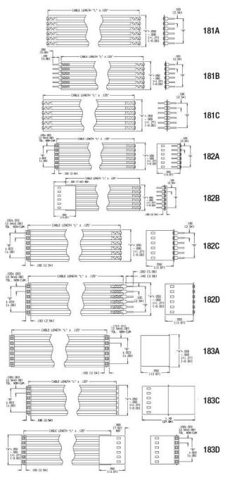
"A"= NO. OF CONDUCTORS x 0.100 [2.54] "B"= (NO. OF CONDUCTORS -1) x 0.100 [2.54]
