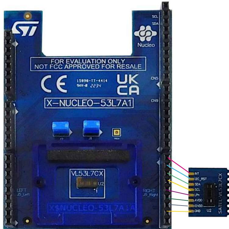
Figure 3. SATEL-VL53L7CX mini-PCB flying wire connection to the X-NUCLEO-53L7A1 expansion board
