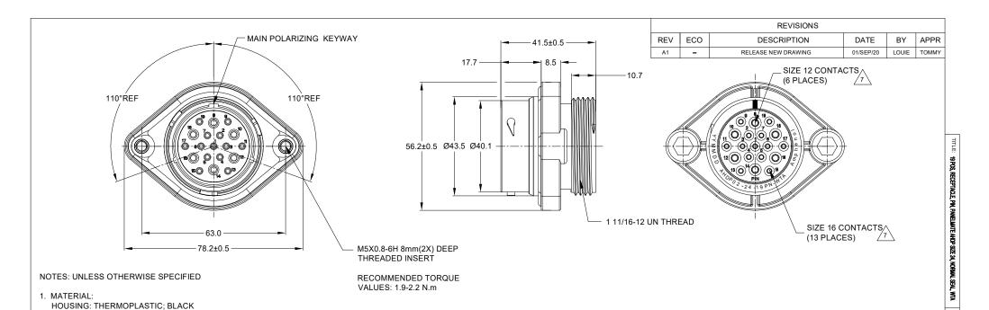
2. MODIFICATIONS: WIDE THREAD ADAPTOR (WTA); STANDARD DIA. WIRE SEAL SEALED PANEL MOUNT
