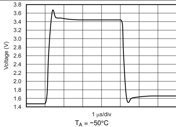
Figure 13. Differential Amplifier: Large-Signal Step Response
