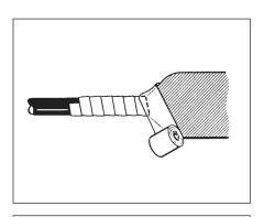
5.2 Fold material over and pull across cable. Continue to wrap using the 60% overlap which in turn will hold down the fold.
