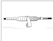
8.11 Overwrap the VM layer with two half-lap layers of #50 tape (highly stretched). Start and end at the center of the repair. The first layer should start going in the same direction as the previous VM layer. Position the #50 tape abutting tightly against both sides of the breather tube as the center is passed. Extend the #50 tape 2" (51 mm) past the ends of the VM tape.
