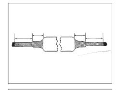
9.2 If the diameter of the lead auxiliary is 1" (25 mm) or more greater than the cable diameter, or if the angle of the transition is steeper than 45°, build up a B sealing tape cone to make a taper of 45° or less between the lead sleeve and the cable.
