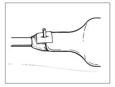
9.4 Starting 4" (102 mm) down the cable sheath, half lap VM tape to at least 4" (102 mm) onto the lead sleeve.
