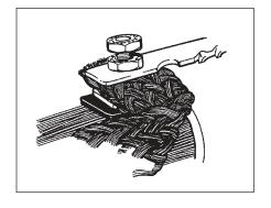
8.9 Starting 4" (102 mm) beyond the #50 tape, apply half-lapped VM tape using moderate tension while wrapping and continue 4" (102 mm) beyond #50 tape at far end. Try to eliminate all but the smallest wrinkles by applying moderate tension.
