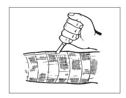
7.2 Use a large screwdriver or similar tool to pry the Armorcast apart. Remove as large a piece as possible. Make additional cuts to remove parts which may be mechanically held.
