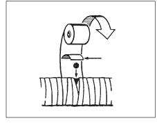
8.13 Following standard wrapping procedures, wrap the entire repair section with Armorcast. Extend the Armorcast 2" (51 mm) past the #50 tape.
