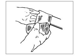
4.2 With slight tension on roll, wrap the entire length of area on the cable with 60% minimum overlaps.
