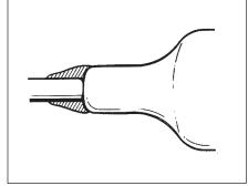
9.3 \*Secure the kit breather tube at the lead to cable junction with a 2" (51 mm) square of VM tape. Prepare the tape making a small slit to allow the tube to fit snugly. Fit the tube into the slot and rub the tape down onto it. If step 9.2 was followed to build a 45° cone, be sure the vent tube provides a clear leak path.
