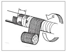
The following wrapping techniques will provide a neat and easy way to cover cable repairs and splices. They will also provide maximum strength by using the 60% overlap method. Changes in wrap diameter may be achieved by using one of the following methods:
