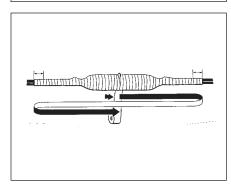
\*When the wrap reaches the breather tube do not cut the tape. Allow the roll to hang. Prepare a 1/2" (13 mm) diameter plug of B sealing tape and a 2" (51 mm) square patch of VM tape. Pull out the breather tube and discard. Press plug into hole. Some plug should remain on the surface. Quickly place and immediately secure VM patch over plugged hole using four layers of highly stretched #50 tape. The #50 tape must completely cover the patch and overlap the edges.
