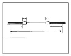
8.10 \* When going over breather tube, do not cut the tape. Split the center of the VM wrap and pull it over the breather tube. Complete the VM wrap.
