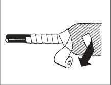
5.3 Additional folds can be made as needed to uniformly cover repair area.
