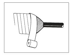
6.2 Slightly relax tension on the roll before folding. Turn over the roll and push back slightly towards work area. This allows the material to relax. Continue using this method until a 60% overlap is reached on the straight cable.
