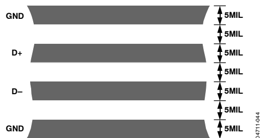
Figure 25. Arrangement of Signal Tracks
