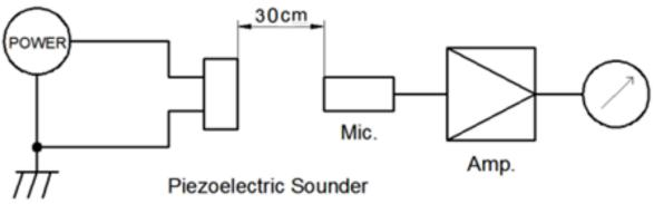
MIC: ND10 Sound Meter or equivalent DC Power Supply: QJ6003S or equivalent
