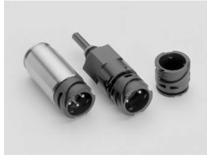
2 to 4-way APD Sensor connector with machined crimp contacts. (Other termination methods are possible). Connector is fixed either by joint flared or over mold.
