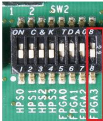
Figure 4-6 USER_DIPSW_FPGA3 location on A10SoC board
