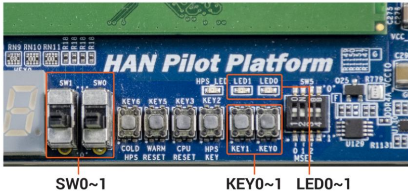
Figure 5-19(5-19) KEYS/SWs/LEDs locations on HAN board
