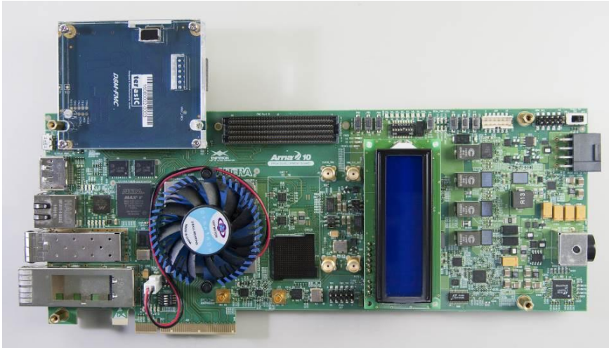
Figure 1-4 Connect the D8M-FMC to A10GFP board's expansion port
