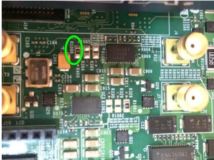
Figure 5-13 Adjust FMC_A VADJ to 1.8V (default) by short R1086
