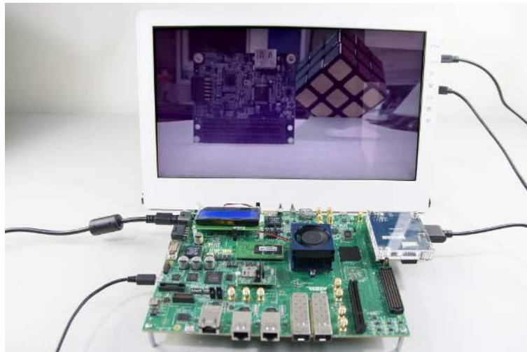
Figure 5-10 A10SoC_D8M_FMC_VIP demonstration running on A10SoC
