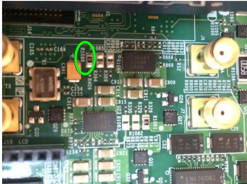
Figure 4-11 Adjust FMC_A VADJ to 1.8V (default) by short R1086
