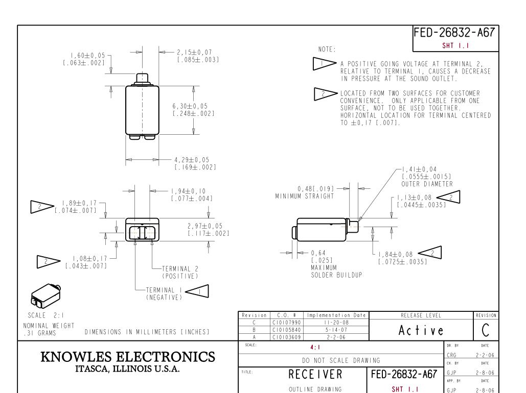
THE FED-26832-A67 IS A FERROFLUID AND TYPE III DAMPED ED RECEIVER WITH A PEAK OF 4dB RELATIVE TO THE SENSITIVITY AT IKHZ UNDER CONSTANT VOLTAGE DRIVE CONDITIONS.
