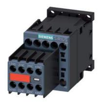
Power contactor, AC-3 7 A, 3 kW / 400 V 2 NO + 2 NC, 110 V AC, 50 Hz 120 V, 60 Hz 3-pole, Size S00 Screw terminal Captive auxiliary switch
