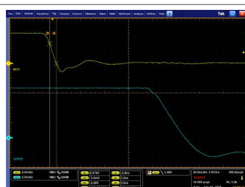
Figure 9-13. PWM Input (yellow) and Driver Output (blue) Falling Edge
