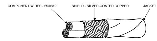
JACKET - LOW OUTGASSING. RADIATION-CROSSLINKED, MODIFIED ETFE
