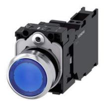
Illuminated pushbutton, 22 mm, round, metal, shiny, blue, pushbutton, flat, momentary contact type, with holder, 1 NO+1 NC, LED module with integrated LED 230 V AC, Spring-type terminal
