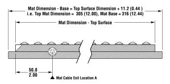
Mat Cable exits on the side indicated by the first dimension in the model number i.e. UM5-1254, Cable exits 12" dimension i.e. UM5-4824, Cable exits 48" dimension
