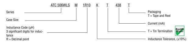
The above part number refers to a 506WLS Series, Case Size M, 1.10 µH inductor, K tolerance (±10%, typ.), with Tin Termination (T), 438 mA, tape and reel packaging.
