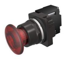
30mm BlackMax, Epoxy Coated Corrosion Resistant Complete Metal Unit Illuminated Push-Pull Operator Full Voltage, 12V AC/DC Incandescent Lamp Mushroom Head Cap Small 1 3/4" (44.5 mm) Plastic, Red 3 Position Pull-Momentary/Push-Maintained UL Listed, CSA Certified NEMA 1,3,3R,4,4X,12,13 & Automotive Standards
