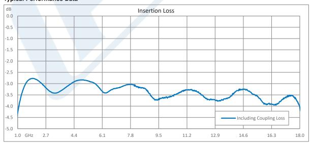
Click the following link (or enter part number in "SEARCH" on website) to obtain additional part information including price, inventory and certifications: 90 Degree SMA Hybrid Coupler from 1 GHz to 18 GHz Rated to 50 Watts PE2CP1144
