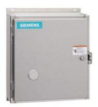
Mechanically held lighting contactor, Contactor amp rating 20Amp 0NC  $\_4NO$  poles, 265-277V 50/60HZ coil, Non-combination type, Encl NEMA type 4X 304 S-steel Water/dust tight noncorrosive
