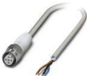
Sensor/Actuator cable, 4-position, PP-EPDM halogen-free, Gray RAL 7035, Free cable end, on Socket straight M12, A-coded, Cable length: 3 m, Hygienic design, With high-grade steel knurl
