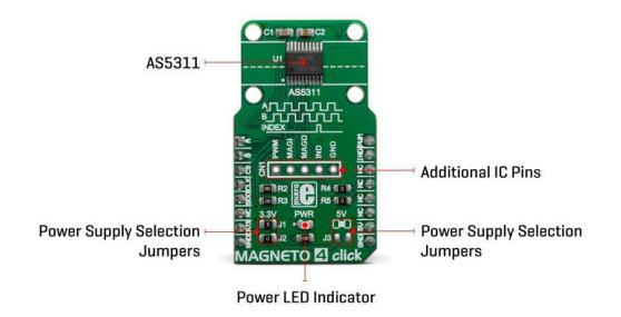
The AS5311 can output the movement data in several different formats: it can either output the bit-string over the serial interface, or by using the 12-bit pulse-width modulated signal (PWM). The pulse width of the PWM signal starts with 1µs and is increased for every 0.488µm. The maximum pulse width is 4095µs, which corresponds to a magnet movement of 2mm.
