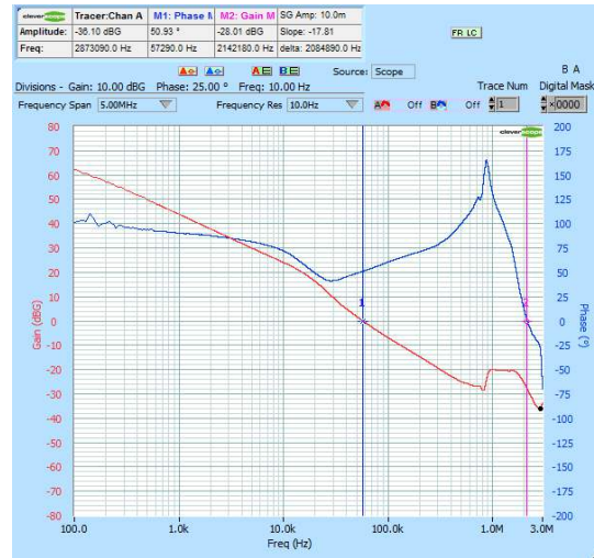
Figure 69. Bode Plot NCV6323FxmLMTW18TBG L = 1.0 μH – COUT = 100 μF
