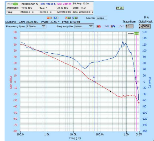
Figure 71. Bode Plot NCV6323FxmLMTW33TBG L = 1.0 μH – COUT = 100 μF
