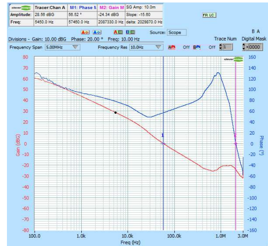
Figure 73. Bode Plot NCV6323FxmLMTW12TBG L = 1.0 μH – COUT = 100 μF
