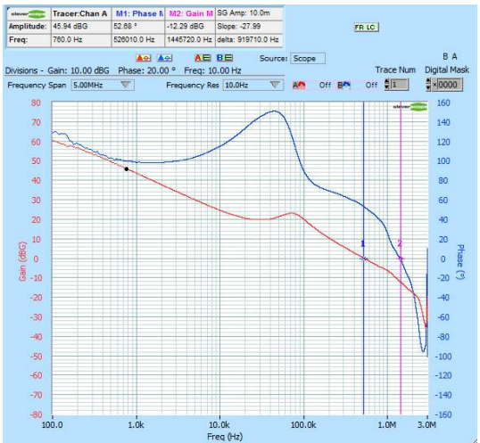
Figure 72. Bode Plot NCV6323FxmLMTW12TBG L = 1.0 μH – COUT = 10 μF
