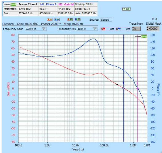
Figure 74. Bode Plot NCV6323F x LMTW10TBG L = 1.0 μH – C OUT = 10 μF
