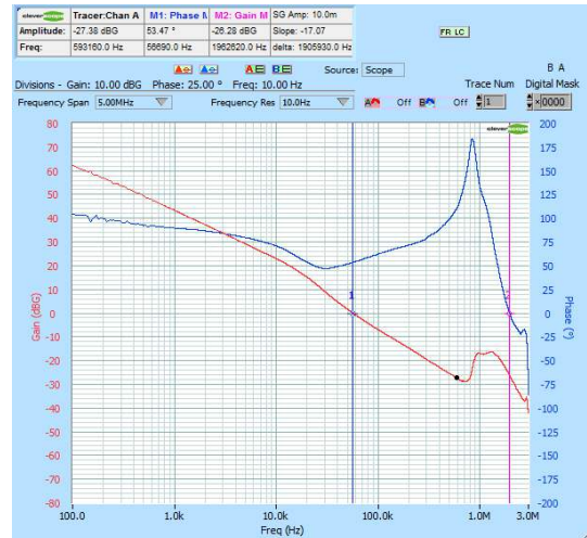
Figure 75. Bode Plot NCV6323F x LMTW10TBG L = 1.0 μH – C OUT = 100 μF
