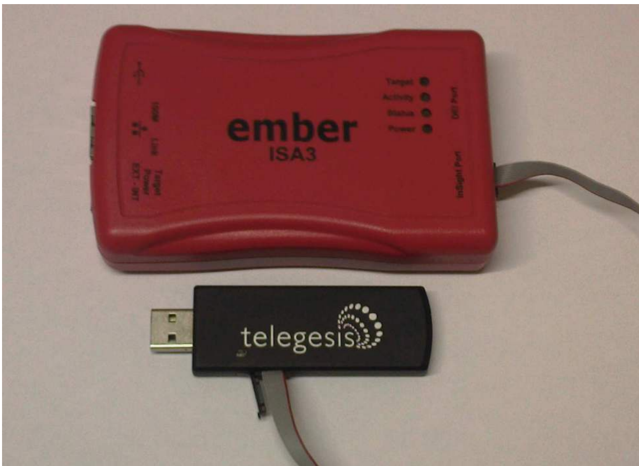
Figure 4: Connecting the ETRX357USB to the Ember ISA3
