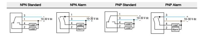
Wiring for the quick disconnect (QD) models is functionally identical.
