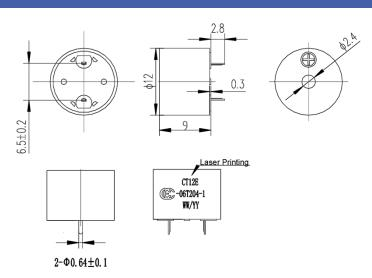
General tolerance =  $\pm 0.5$  mm and all measurements in mm unless otherwise noted.
