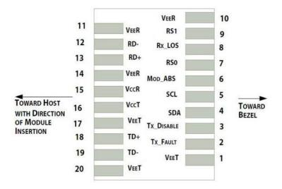
Pin-out of connector Block on Host board
