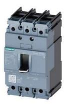
circuit breaker 3VA5 UL frame 125 breaking capacity class S 25kA @ 480 V 3-pole, line protection TM210, FTFM, In=40A overload protection Ir=40A fixed short-circuit protection Ii=10 x In UL489 SB (naval), 50 deg. cel. cable connection on both sides
